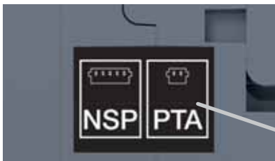
Integrated PTA output contact Output contact dedicated to the overload prealarm.
